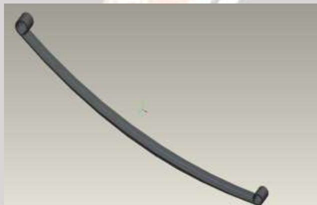
Fig. 6.1 Model of EN47 Leaf Spring in Pro-E 4.0
