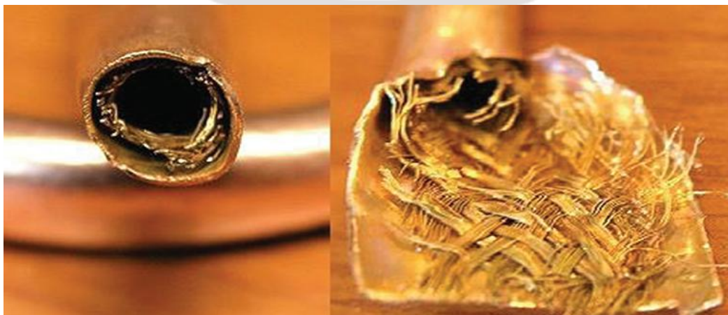
Fig 1. Cross-section of Mesh Wick Structure of Heat Pipe
