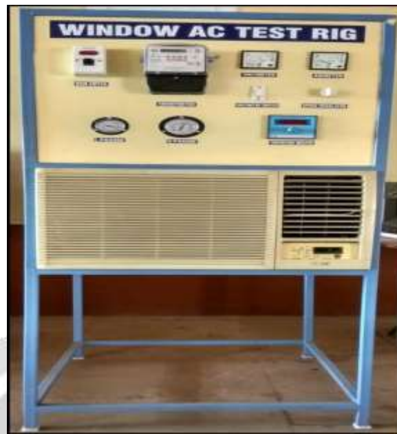
Fig.-2: Window Air Conditioning Test Rig 2.2 Refrigerant charging:
