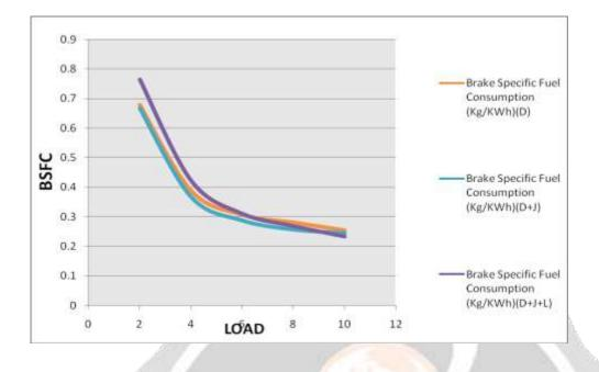
Diesel + Jatropha + LPG has highest bsfc as compared to diesel, diesel + Jatropha for load up to 4 kg. After that it is decreasing slightly. Maximum BSFC of tri fuel is 0.764 at 2 kg load and minimum at 10 kg load is 0.234
