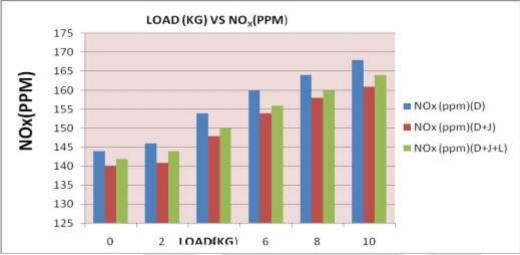
The result shows that, as blending increases,  $NO_X$  emission was continuously decreased at all load. As compared to diesel fuel,  $NO_X$  emission from blends fuels was less.
