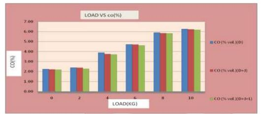
the variation in CO emissions with load.CO emission is increase as load on engine increase at all speed. CO emission decreases as blending increase. Value of CO for tri fuel blend is 6.18 for tri fuel.
