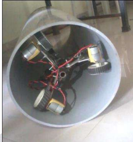
Fig:- Leak Detection Robot
