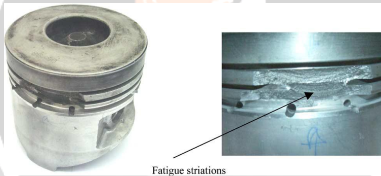
Fig. 7- Engine piston with damaged grooves: (a) piston; (b) detail of damaged grooves.
