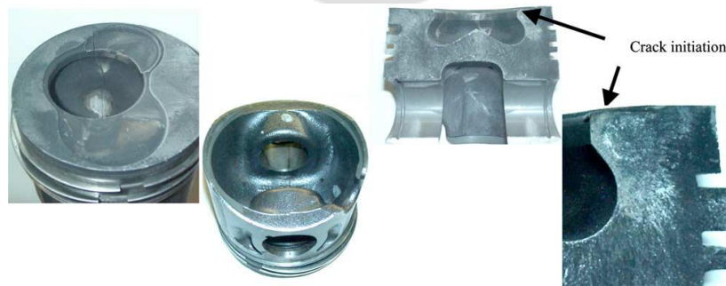
Fig.5 - Diesel engine piston with a crack from one side of the pin hole to the other pin hole going through the head of the piston
