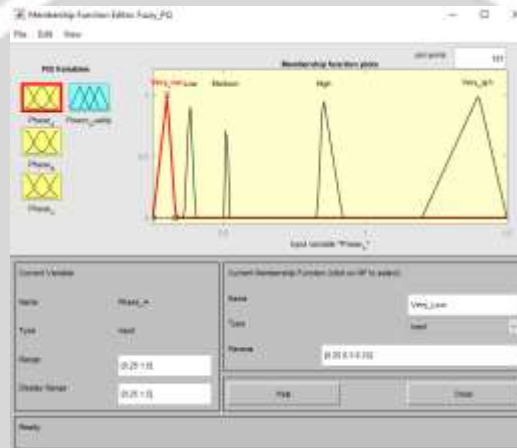
Fig-3: Fuzzy membership function for input voltages Va, Vb and Vc RMS values
