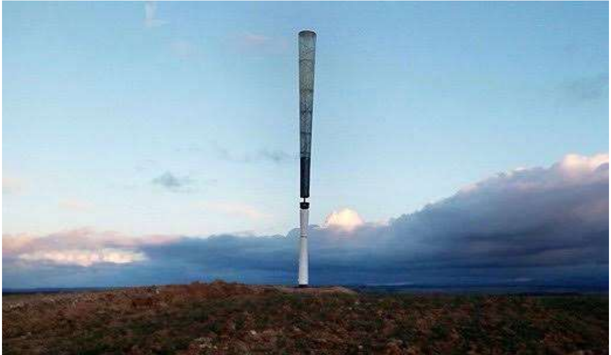
Fig no. 1 vortex windmill (vortex free standing structure)
