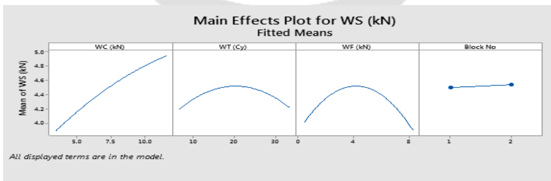
Fig. 5 Main effect plot for the weld strength
