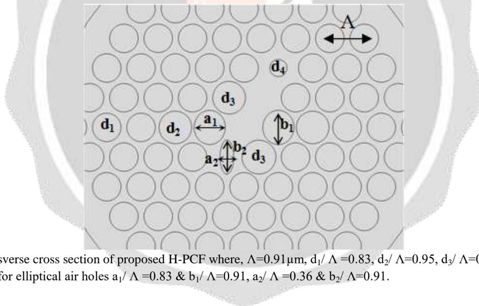
Fig. 1 Transverse cross section of proposed H-PCF where,  $\Lambda = 0.91 \mu\text{m}$ ,  $d_1/\Lambda = 0.83$ ,  $d_2/\Lambda = 0.95$ ,  $d_3/\Lambda = 0.9$ ,  $d_4/\Lambda = 0.5$  and for elliptical air holes  $a_1/\Lambda = 0.83$  &  $b_1/\Lambda = 0.91$ ,  $a_2/\Lambda = 0.36$  &  $b_2/\Lambda = 0.91$ .
