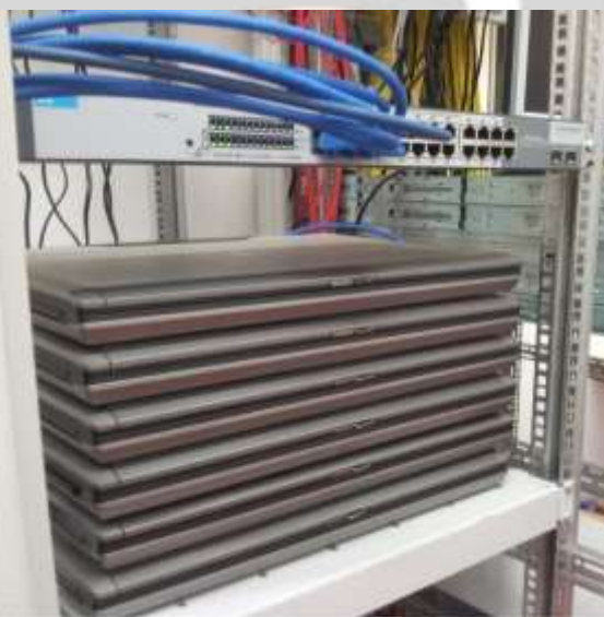
Fig-1:A Beowulf cluster constructed of six laptops and an old switch.
