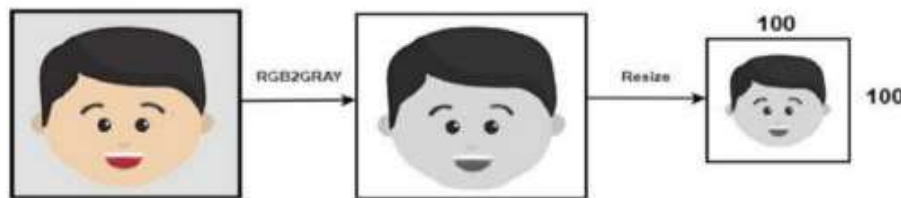
Fig-4: Converting An RGB Image To A Gray Scale Image Of Size:100 X 100
