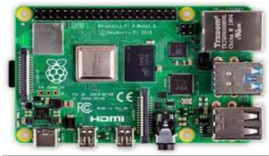
Fig1. Circuit Board of Raspberry Pi IV
