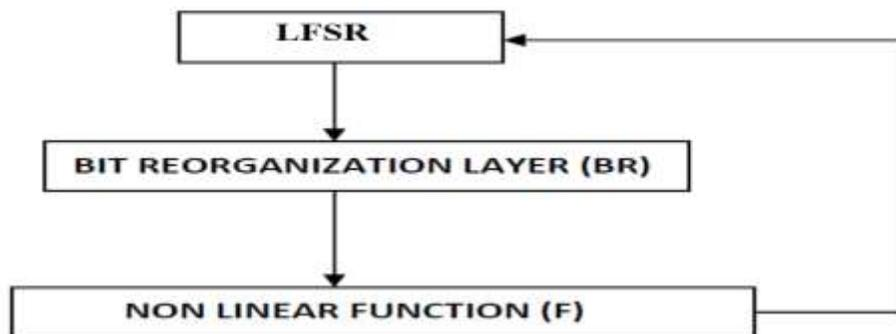
**Fig.2 Work flow of ZUC Stream Cipher**
