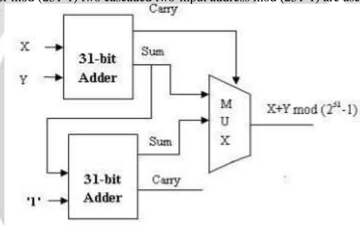
Fig. 4 The Architecture of Adder mod  $(2^{31}-1)$ .
