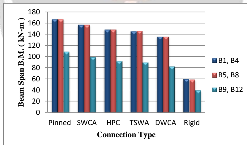
Fig-9: Beam Span Bending Moment for 1.5DL+1.5LL
