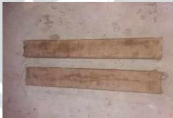
Fig 4 Beam wrapped using jute fiber sheet
