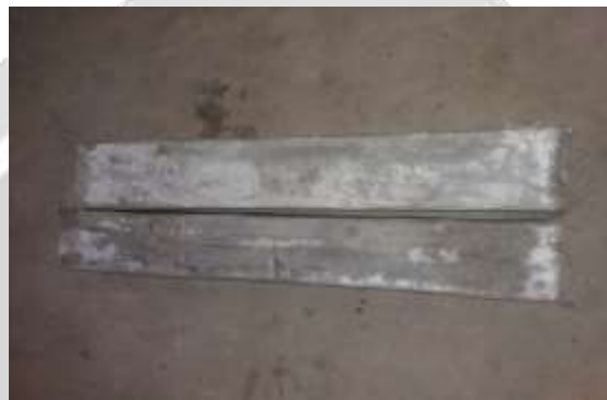
Fig 3 Beam wrapped using jute fiber sheet
