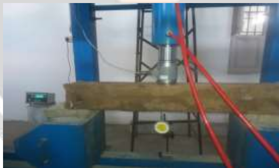
Fig 7 View of load applied on wrapped jute fiber specimen
