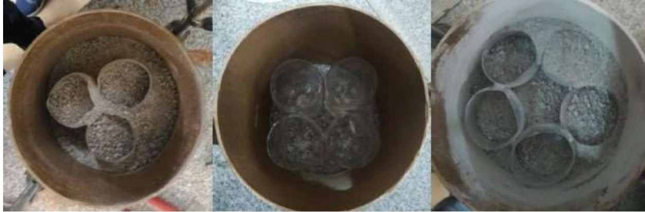
Figure -1: Test Configurations Within CBR Moulds.
