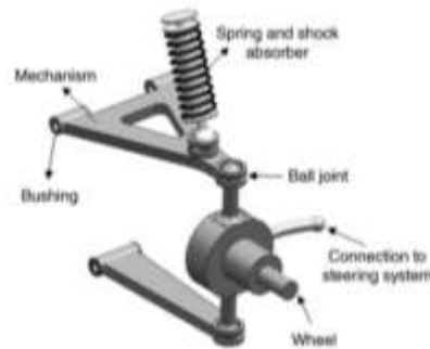
Figure 1.2 Main parts of a typical suspension system
