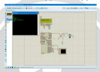
The motor stops running when the user account has insufficient balance for the payment of tax. The LCD available will display "NO BALANCE".
