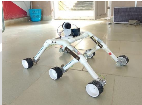
Fig 2: Rocker Bogie System
