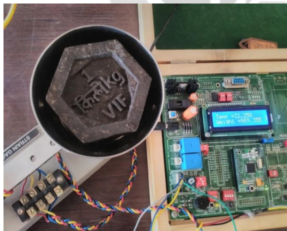
Figure 4.2: Display temperature and force on LCD
