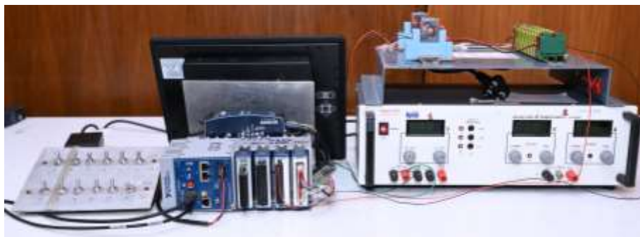
Fig -5: NI cDAQ-9136 simulation bench setup for FN
