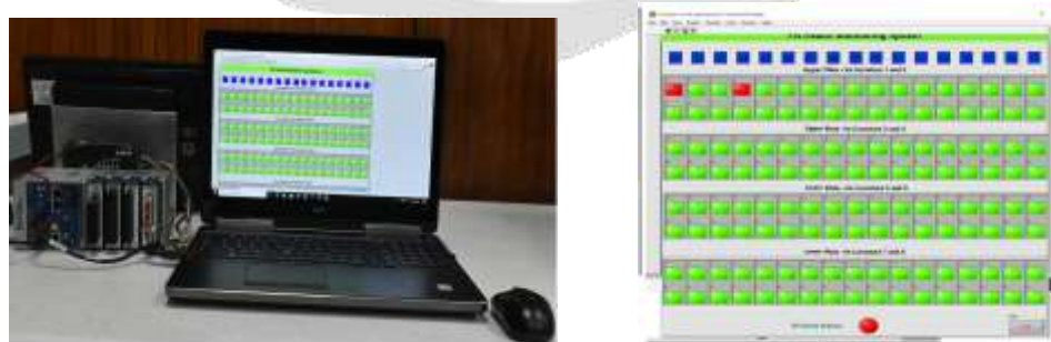
Fig -8: Real-Time health monitoring setup and system display without stress(Green) & With Stress (Red)
