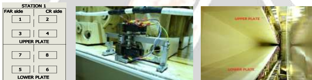
Fig -2: Schematic diagram of Curvature sensor assembly mounted on nozzle plate
