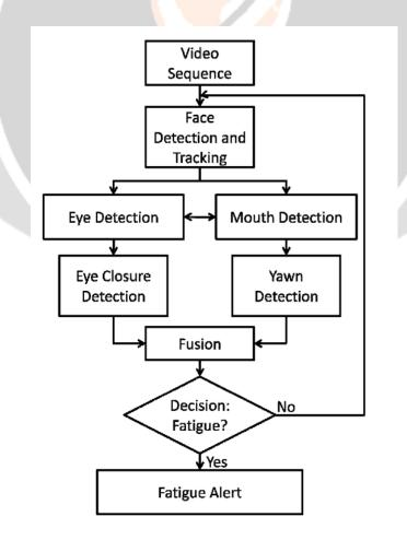
**WORKING:** - The Driver Drowsiness Detection (DDD) system is a sophisticated solution designed to monitor driver alertness in real-time, enhancing road safety by preventing accidents caused by fatigue. The system begins by capturing video streams using high-resolution cameras positioned within the vehicle. These cameras are equipped with night vision, ensuring consistent
