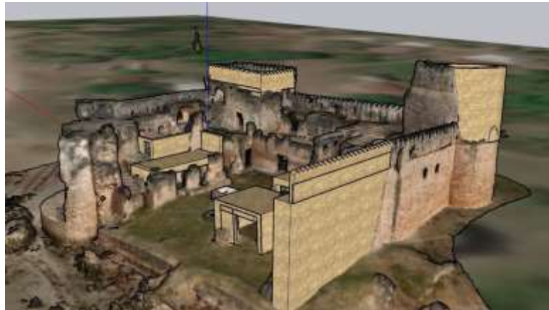
Fig -3: Kilwa Kisiwani fortress model rendered in SketchUp enables interactive visualization and measurements.
