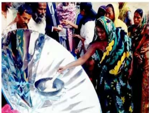
Fig.3: Solar cooking by a paraboloidal concentrator
