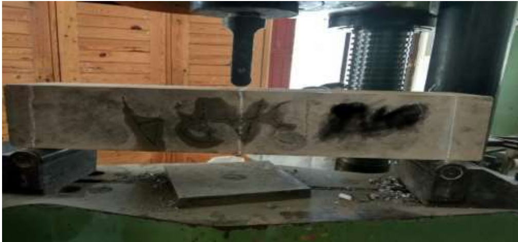
Fig. 2 Failure of Flexure Specimen
