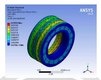
As the induced stress is well below the permissible limit the part is safe
