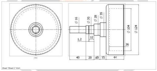
Material of Input drum shaft allowable stress =  $110 \text{ N/mm}^2$  $\Rightarrow$  T design = 0.475 Nm
