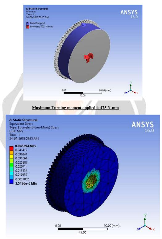
As the induced stress is well below the permissible limit the part is safe
