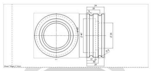
Material of Roller EN9 allowable stress =  $90 \text{ N/mm}^2$  $\Rightarrow$  T design = 0.475 Nm
