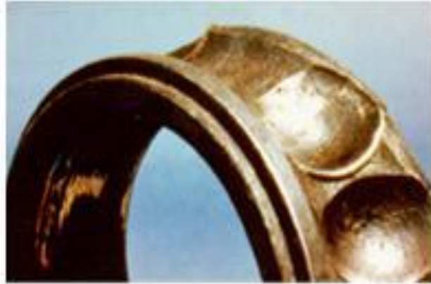
Figure 11 Plastic deformation on an inner ring raceway produced by overloading
