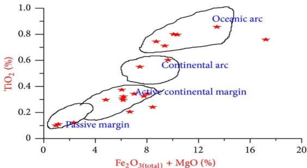
**Fig. 2:** Bivariate plot of  $\text{TiO}_2$  versus  $(\text{Fe}_2\text{O}_3+\text{MgO})$  diagrams for sandstones.
