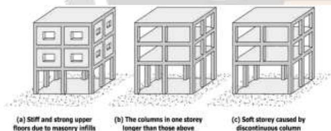
**Fig. 1: Example of soft storey**
