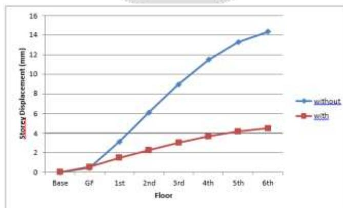
Fig. 7.3: Storey Displacement in no soft storey at X direction
