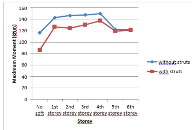
Fig. 7.1: Bending Moment (KN-m)
