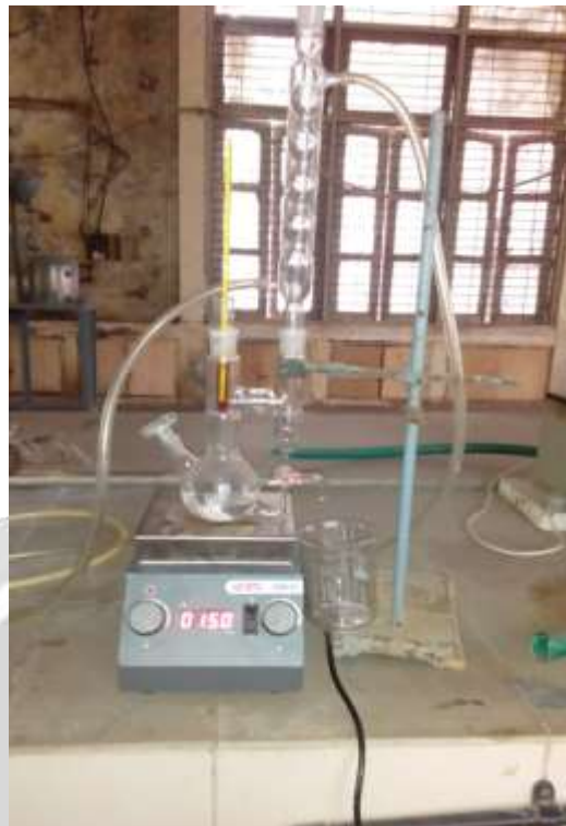
Figure 1: Experimental Set - up for vapour - liquid equilibrium in laboratory
