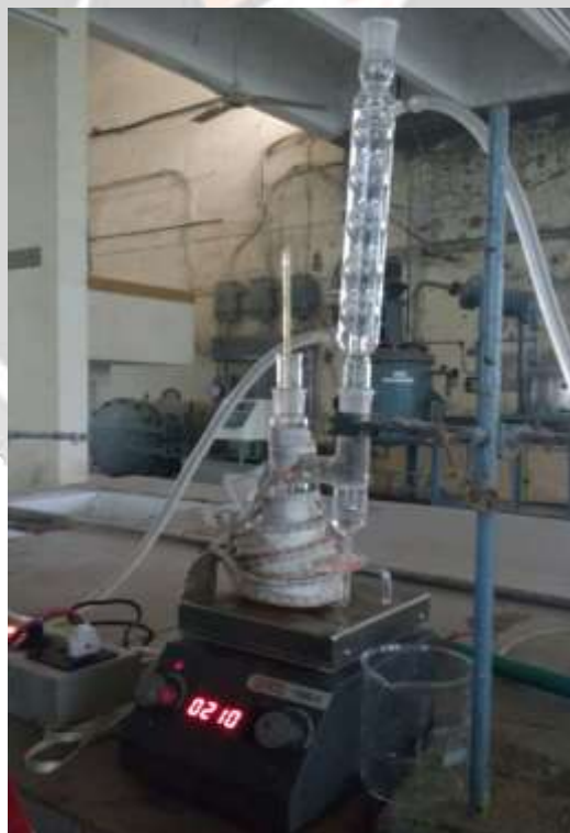
Figure 2: Experimental Set - up for vapour - liquid equilibrium in laboratory
