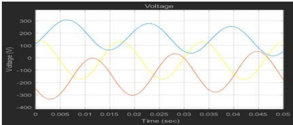
**Figure 6: Voltage Response Waveform Simulink DGP-1 Module for Non-Linear Load**
