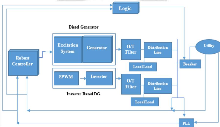
Figure 1: Micro-Grid Equipped with the Proposed Robust Controller
