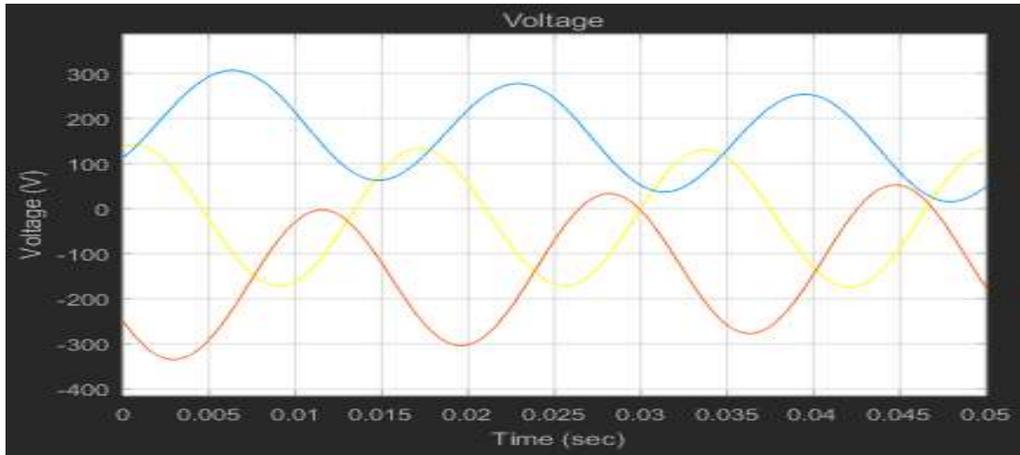
**Figure 3: Voltage Response Waveform Simulink DGP-1 Module for Linear Load**
