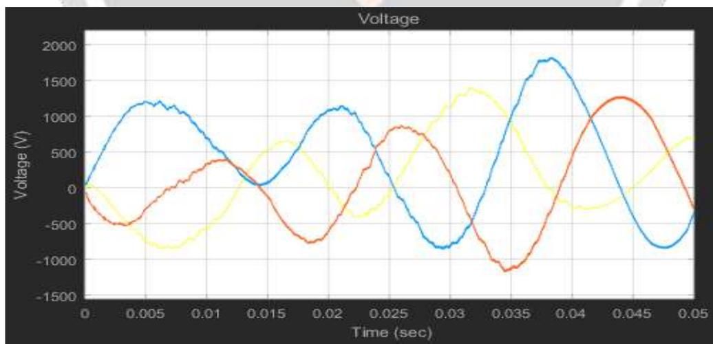
**Figure 8: Voltage Response Waveform Simulink PV Module for Non-Linear Load**
