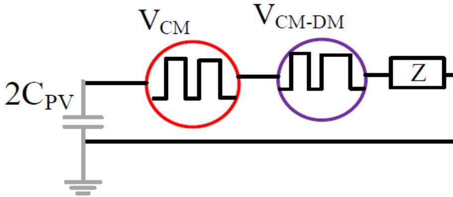
Figure 9: Single phase equivalent circuit using the common-mode voltage model TL-TPC-MLI DM to CMV impact via VCM-DM is equivalent to -VDM/2 in this example.
