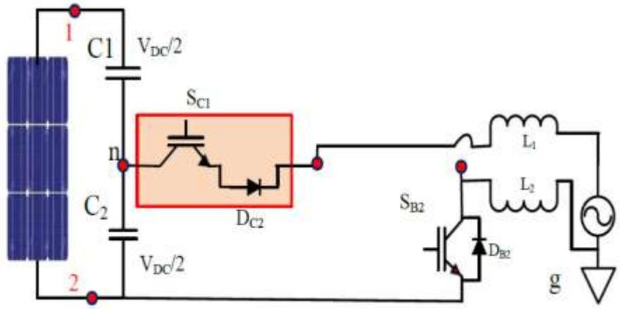
Figure 4:  $1-\theta$   $V_O = V_{PV}/2$  Mode-2 of operation for TL-TPC-MLI
