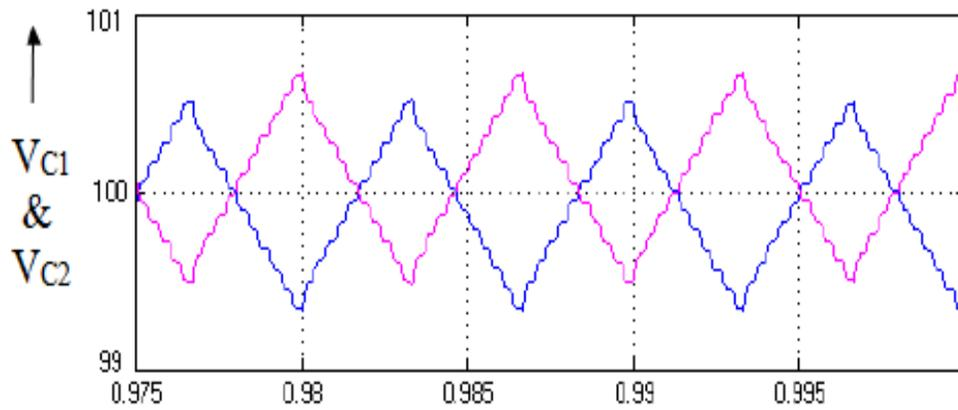
Figure 18: DC-link capacitor voltage profile simulation results for Ma=1
