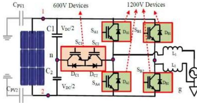
Figure 1: Single-phase t-type transformer less NPC- MLI
