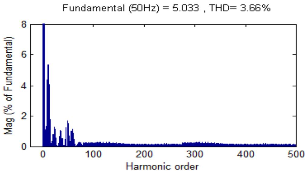
Figure 17: Simulation results for current THD Spectra at  $M_a=1$
