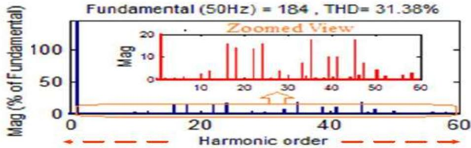
Figure 14: Simulation results for voltage harmonics Spectrum at Ma=1
