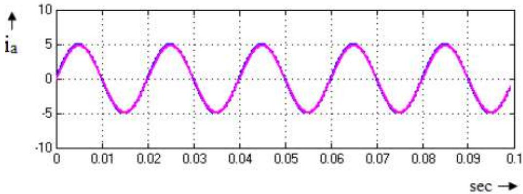
Figure 16: T-Type transformer less inverter output current simulation results for  $M_a=1$  and  $f_o=50$  Hz.
