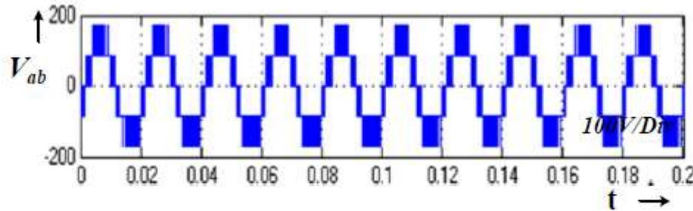
Figure 12: For  $M_a=1$ ,  $f_o = 50$  Hz, and  $V_{dc}=200$  V, of single phase T-Type transformer-less inverter output voltage.
