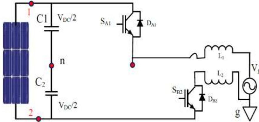
Figure 3:  $1-\theta$   $V_O = V_{PV}$  Mode-1 of operation for TL-TPC-MLI
