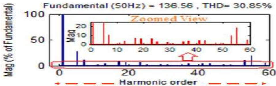
Figure 13: Simulation results for voltage harmonics Spectrum at  $M_a= 0.6$
