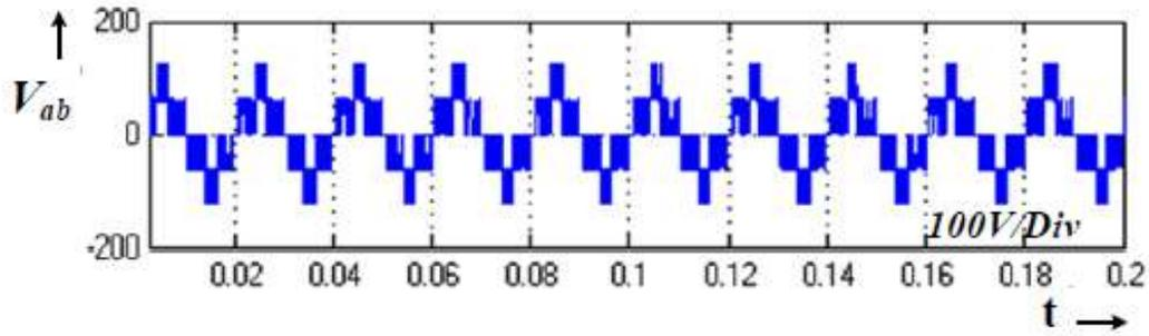
Figure 11: Single phase T-Type transformer-less inverter output voltage for  $M_a=0.6$ ,  $f_o = 50$  Hz, and  $V_{dc}=200$  V.
