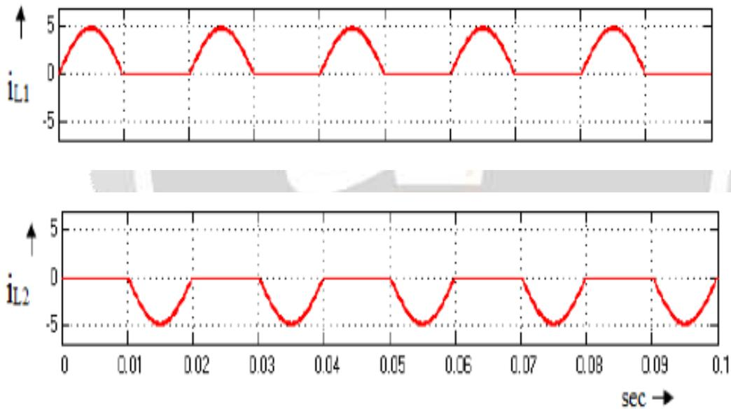
Figure 15 Simulation results for single phase T-Type transformer less inverter inductor current ( $i_{L1}$  to  $i_{L2}$ )
