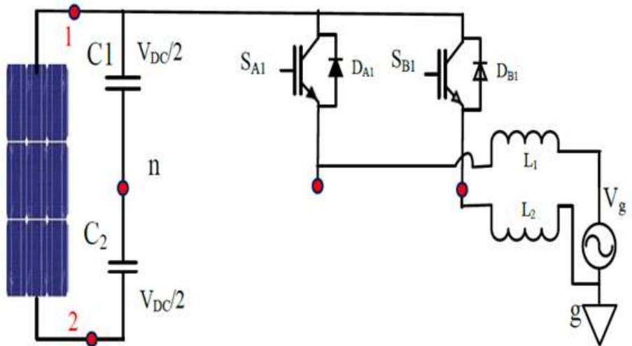
Figure 8: 1- $\Theta$  TL-TPC-MLI operating mode-6, leakage current is freewheeled
