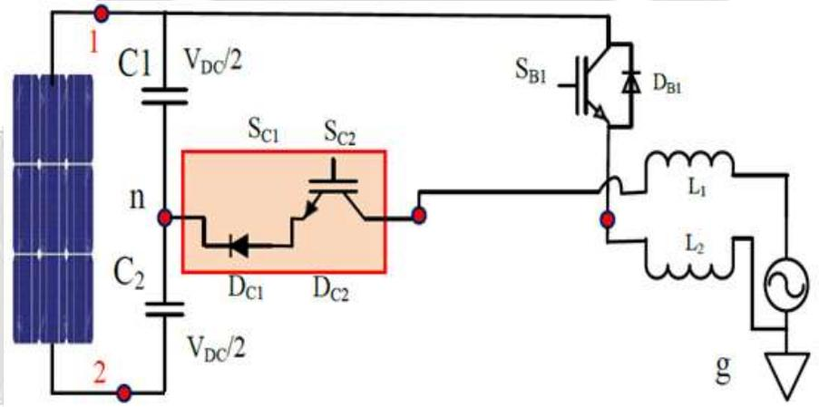
Figure 77: 1- $\Theta$  TL-TPC-MLI operation mode-5:  $V_O = -V_{PV}/2$
