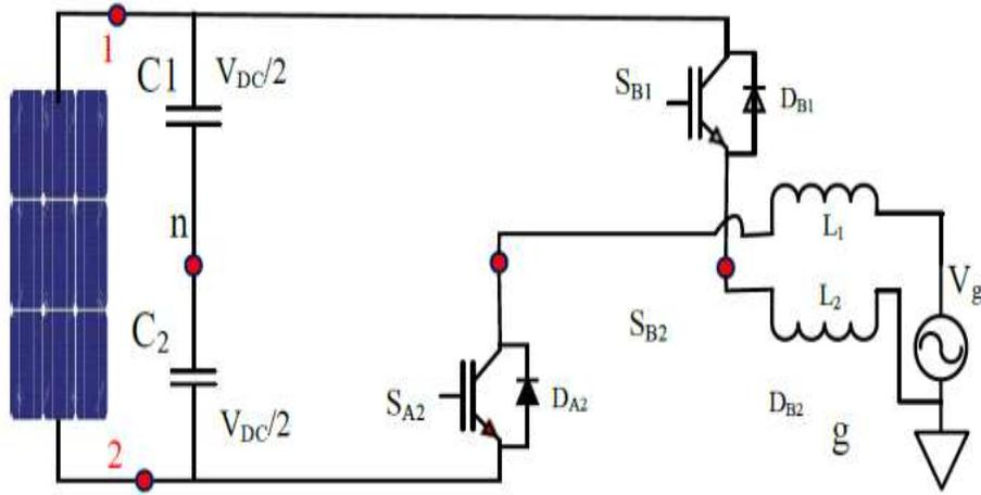
Figure 6: 1- $\Theta$  TL-TPC-MLI operation mode-4:  $V_O = -V_{PV}$
