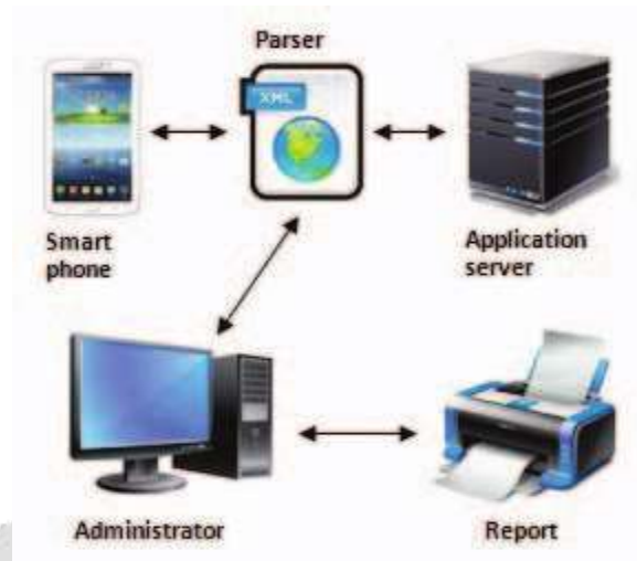
Fig. 1. Architecture of smartphone attendance system.
