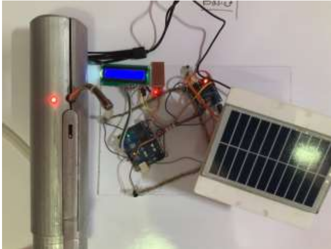
Figure-5.2 charging of smart drinking water dispenser using solar energy.
