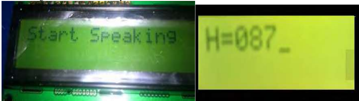
Fig.4 shows the initial value displayed on resetting the voice recognition unit.
