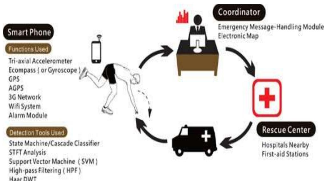
Fig.3. Architecture of the proposed fall accident detection and rescue system.
