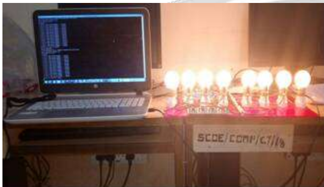
The above figure shows the output for command given from android application. The given hardware is connected to server via internet.
