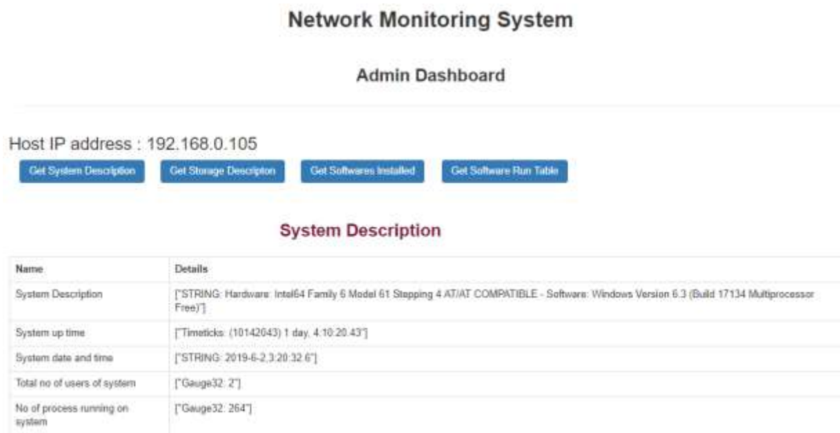
Figure 3.3: A sample of data returned from successive SNMPGET commands for system description on a Windows host
