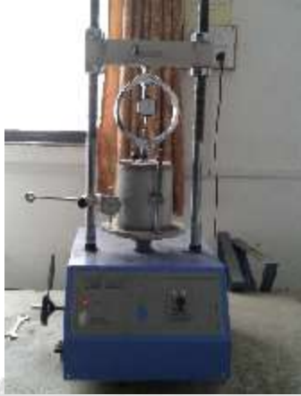
Fig -1: CBR Test Assembly
