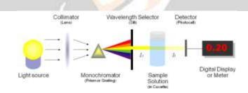
Fig 2: Basic structure of spectrophotometer (illustrated by Heesung Shim)
