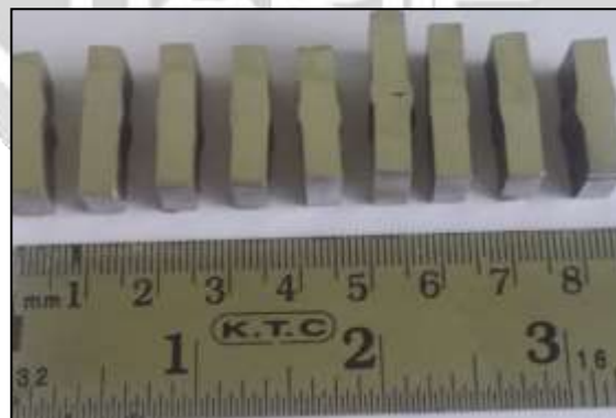
Fig.9 Micro hardness Sample of TIG
