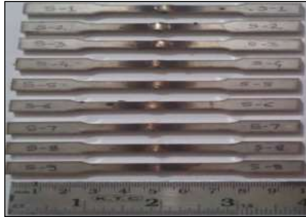
Fig.4 Tensile Test Sample for SMAW Joints
