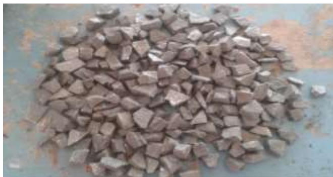
Fig No.3- Shabath Stone Waste, Manual Cutting and Preparation of Aggregate
