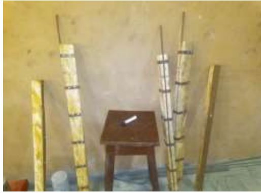
Figure -6: Steel Reinforced Beam Samples
