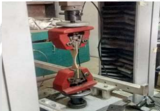
Figure -5: Tensile Test for Ayin Timber in UTM
