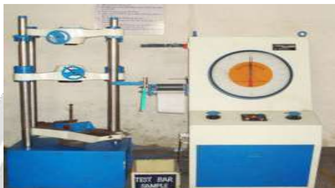
Fig 2. Process Setup for Tensile Test
