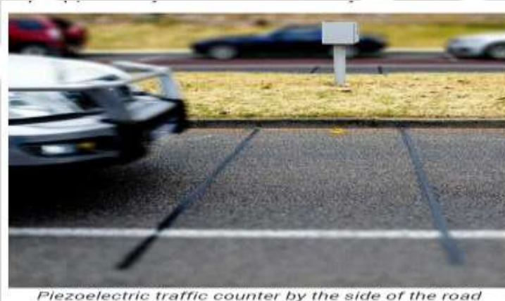
Fig-1. Piezoelectric detector for vehicles.
