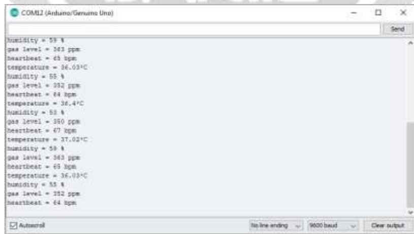
Fig -5: Serial monitor reading of Lifi receiver
