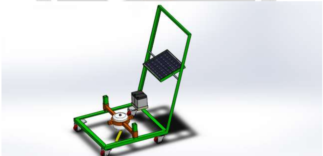
Fig -1 view of solar grass cutter
