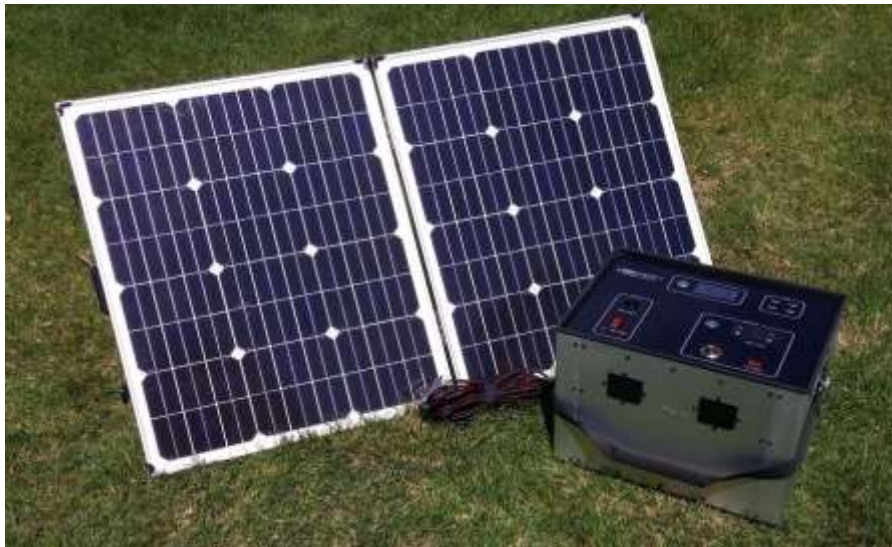
Fig. Battery unit with solar panels
