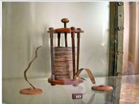
A voltaic pile, the first chemical battery
